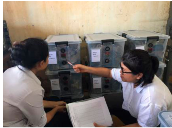
FIGURE 6. Learning how to read the hygrometers on the Dryboxes to track RH and temperature. Photo Tuol Sleng Genocide Museum.
